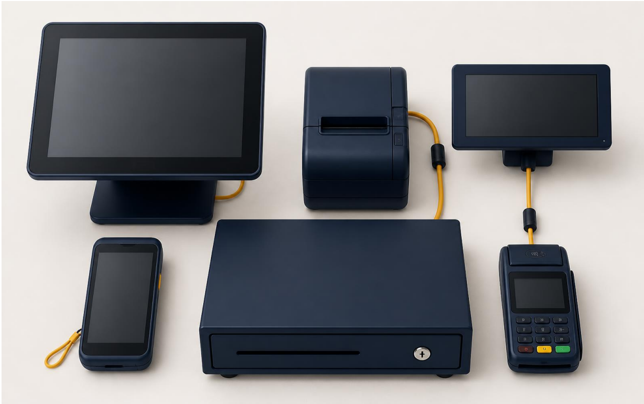
A complete setup: register, receipt printer, cash drawer, customer display, handheld and payment terminal.
